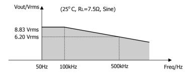
the amplifier are Slew Rate and the Heat Extraction when a signal with high amplitude is input. Along with the frequency increase of the input signal, the working current and the power consumption of the instrument without loads as well as the signal distortion will be increased that may heat the amplifier and reduce the performance. Thus, we set limits on the relationships between the frequency and the amplitude of output signals which have high amplitude.
