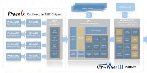
DS70000 series digital oscilloscope is equipped with "Phoenix" chip set, which delivers a max. of **20 GSa/s sample rate** and **5 GHz bandwidth** to better achieve signal fidelity, cover more application scenarios, and cater to the diversified application demands of the complex test system in the industry and R&D fields.
